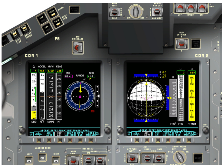
Commander Front panel with the HSI and ADI displays
